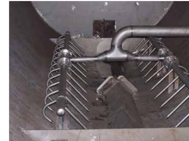
Fig. 16 Sand Jet Nozzle Header
