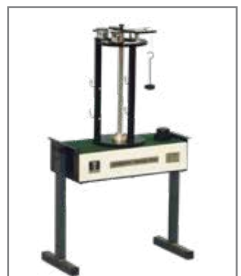
SDB-20 Deflection of Unsymmetrical Beams
