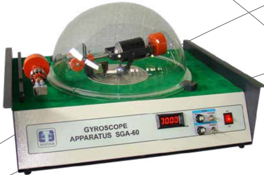
SGA-60 Theory of Machine Teaching Equipment Gyroscope
