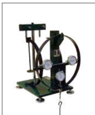
SDB-30 Deflection of Curved Beams
