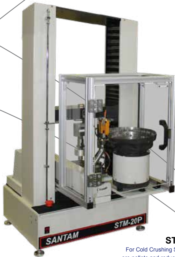
Single Pellet Crush Strength of Formed Catalyst Shapes Bulk Crush strength of Catalysts
