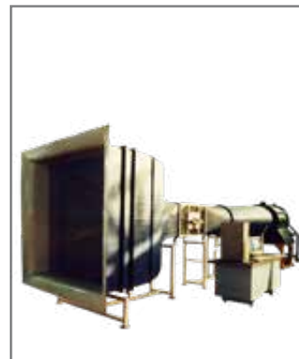
SWT-30 Wind Tunnel Computrized, 40x40 cm Test Section, 30m/Sec
