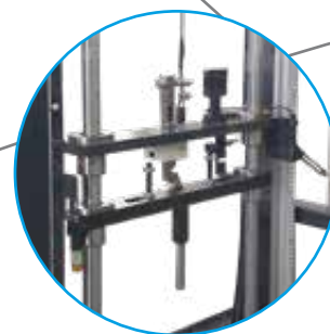
SDWT-100 Drop weight Testing Machine ASTM D7136/D7136M-15 100 J Capacity
