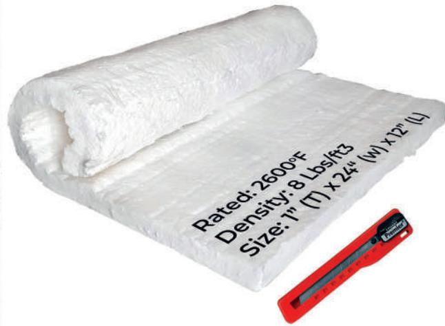
Ceramic fiber blankets made of strong ceramic fibers are good insulators at temperatures higher than 1200 to 1600 degrees Celsius. Among the salient features of ceramic blankets are good flexibility, low thermal conductivity, resistant to thermal shocks and relatively easy to use.
