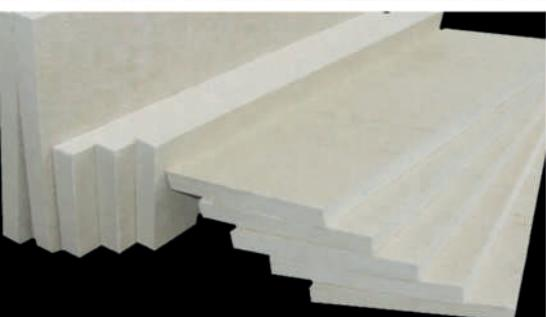
Ceramic fiber insulating boards are made of compressed ceramic fibers and are suitable for temperatures 1200 to 1430 degrees Celsius. Among the salient features of ceramic boards are insulation, low thermal conductivity, resistance to thermal shocks and some chemicals, and good cutting ability.
